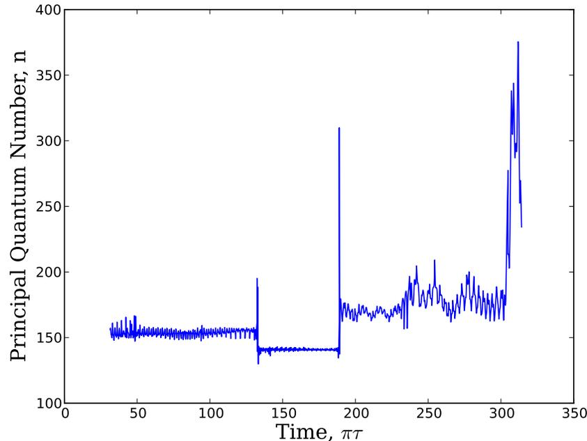
FIG. 2. Plot of the principal quantum number  $n(t)$  as a function of time for one of our recombination events. On the  $x$ -axis is scaled time,  $t_* = \pi\tau$ , where  $\tau$  is the number of trap cycles. A plateau in  $n(t)$ , of about 30 ns duration, corresponds to transient  $\bar{\text{H}}$  formation.
