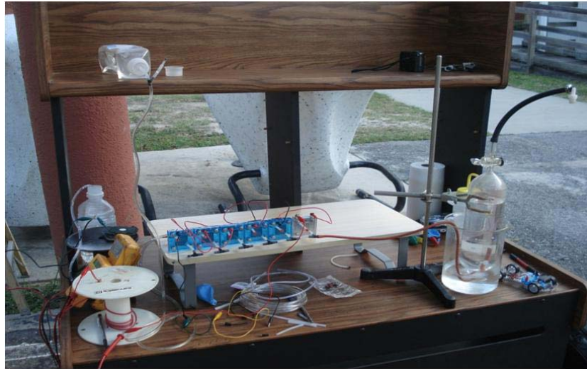
Figure 1: Hydrogen production set up using solar PV electrolysis
